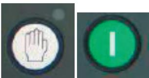
△ Attention: when you do an emergency starting the engine will not stop neither positioning the starting key in OFF position, nor using the emergency stop button “mushroom” type.
